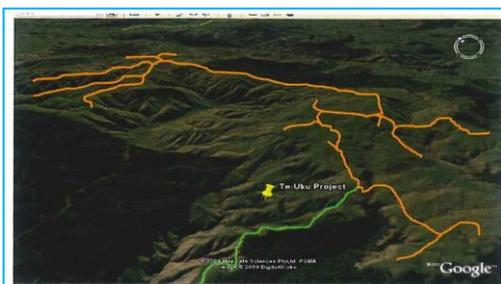
**Figure 4:** Re-alignment and widening of existing paper road to form main access Road A (green), and construction of new turbine access roads (orange) (Google Earth 2009)
