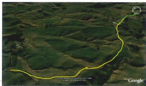
**Figure 5:** Re-alignment and widening of existing Plateau Rd (yellow) and existing paper road (green) to form main access Road A. (Google Earth 2009)
