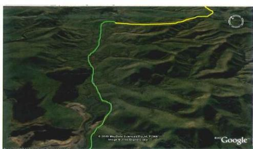
**Figure 6:** New access road (green) from Te Mata Quarry entrance to existing Plateau Rd (yellow) to form main Access Rd A. (Google Earth 2009)
